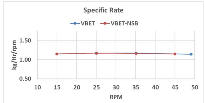
Figure 11. Specific rate as a function of screw speed.
