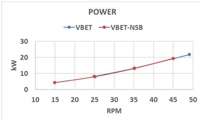
Figure 9. Power required as a function of screw speed.
