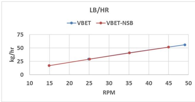
Figure 8. Rate as a function of screw speed.
