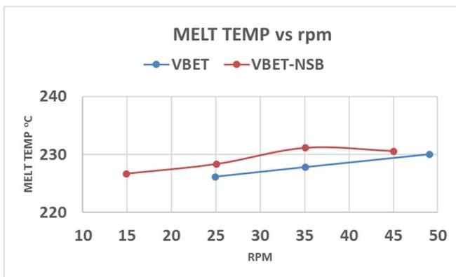
Figure 10. Discharge temperature as a function of screw speed.
